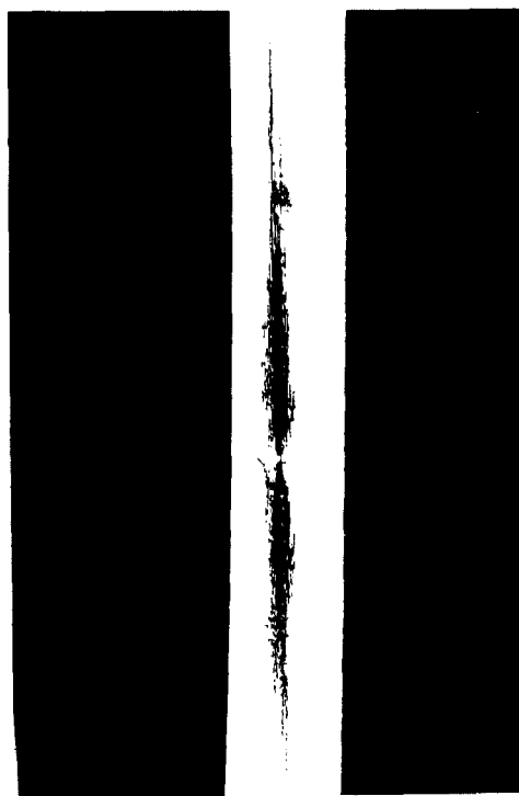
Figure 2 Photograph of electrochemically reduced ram-extruded PTFE rod, \times 2.5 .
